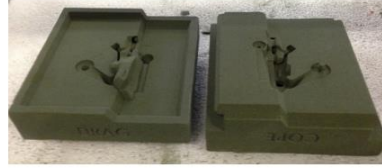
Printed Sand Mold (source: PennState University)
