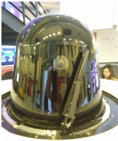
Google's self-driving car unit Waymo showed last year how it uses small windshield wipers to clean the LIDAR domes on its cars
