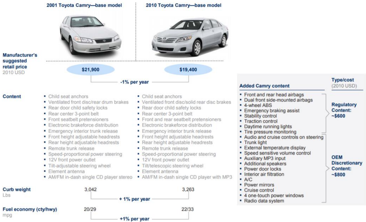
FIGURE 15: TOYOTA CAMRY FEATURES AND CURB WEIGHT FOR 2001 AND 2010 BASE MODELS
