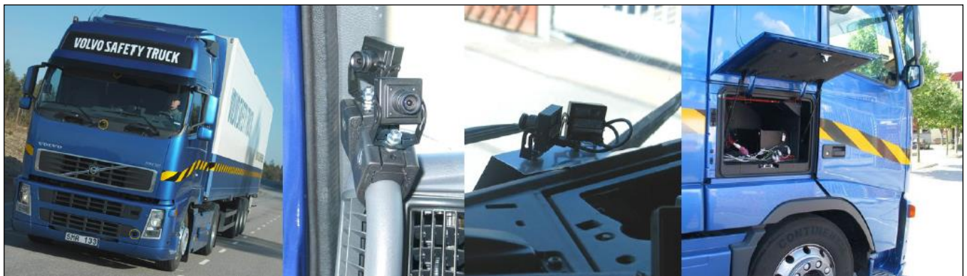
Figure 22: Volvo FH12, Cameras, and Location for System Installation in Side Compartment
