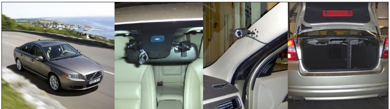
Figure 23: Volvo S80, Cameras, and Logger Installation in Luggage Compartment
