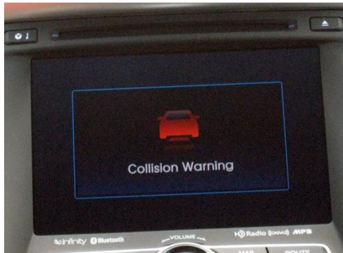
FIGURE 2: EXAMPLE OF DRIVER INTERFACE IN INTEGRATED LIGHT VEHICLE (FCW VISUAL IN CENTER STACK)
