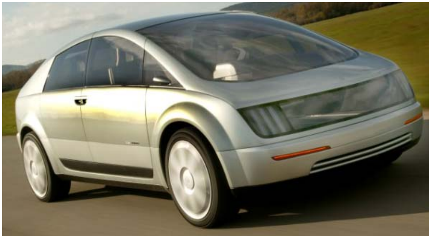
Figure 17 General Motor's Hy-Wire prototype fuel cell car recently drove the roads in Monaco. The Hy-Wire not only demonstrates advanced power technology, but also how vehicles can be redesigned. Note that the Hy-Wire's propulsion components are all underneath, and there's no hood in front of the car. -Photo courtesy of General Motors Corporation
