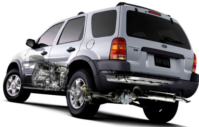
Figure 14 This illustration shows the powertrain innards of the 2004 Ford Escape Hybrid, the first HEV aimed at the popular sport utility vehicle segment. It will deliver nearly 40 mpg in city driving without sacrificing acceleration performance or cargo capacity. - Photo courtesy of Ford Motor Company
