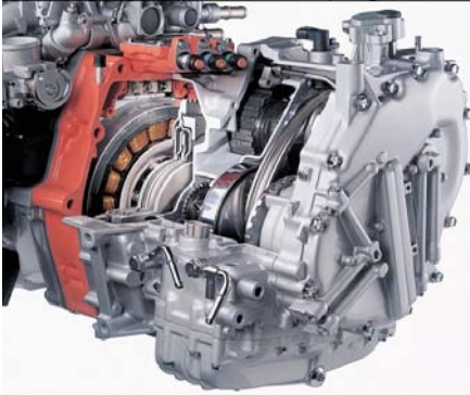
Figure 15 This picture shows a cutaway of the Honda hybrid electric vehicle engine. - Photo courtesy of Honda
